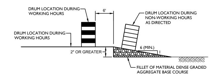
THE CONTRACTOR SHALL BE RESPONSIBLE FOR PREPARING A TRAFFIC DETOUR PLAN TO BE USED DURING PAVING OPERATIONS AND OBTAINING APPROVAL FROM THE TOWNSHIP POLICE DEPARTMENT AND TOWNSHIP ENGINEER. THIS TRAFFIC CONTROL PLAN SERVES FOR USE WHEN THE CONTRACTOR IS ENGAGED IN CONCRETE WORK, SANITARY SEWER REPAIR, PAVEMENT BASE REPAIRS, ETC.
