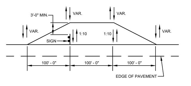
STEEL U-POST GRADING DETAIL
