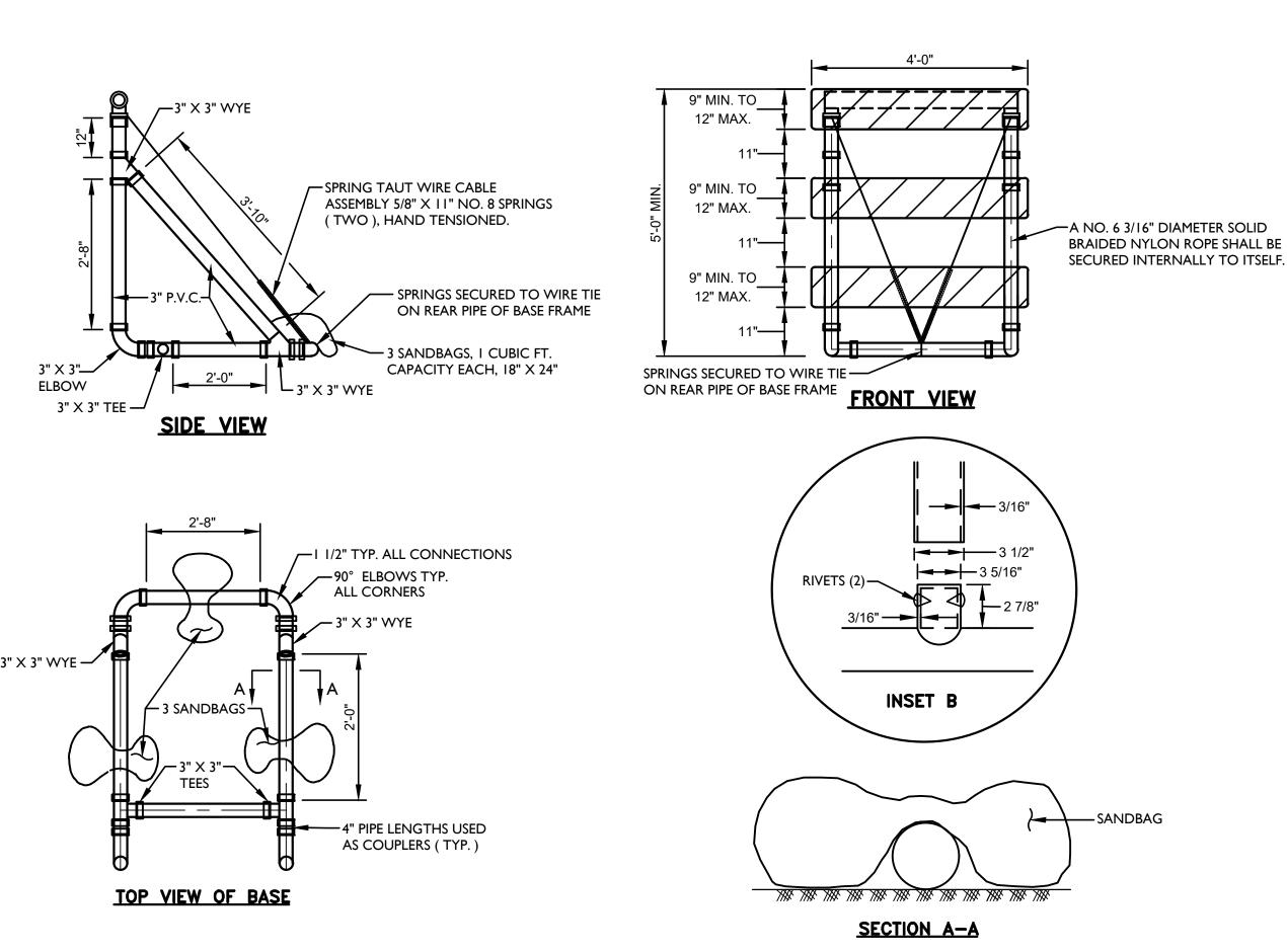
PIPE SHALL BE WHITE PVC SCHEDULE 40 ASTM D 1785 OR PVC, SDR-26 ASTM D 2241. FITTINGS SHALL BE WHITE PVC OR ABS OF MATCHING WALL THICKNESS AND INSIDE DIAMETER AND MEETING THE MATERIALS, REQUIREMENTS AND TESTING SECTIONS OF ASTM D 2466 FOR PVC AND ASTM D 2468 FOR ABS. ALL JOINTS SHALL BE SLIP FIT AND NOT THREADED OR CEMENTED. PVC FITTINGS MEETING ASTM D 2665 WILL ALSO BE ACCEPTABLE. PVC OR ABS MATERIAL SHALL BE ULTRAVIOLET LIGHT STABILIZED.
