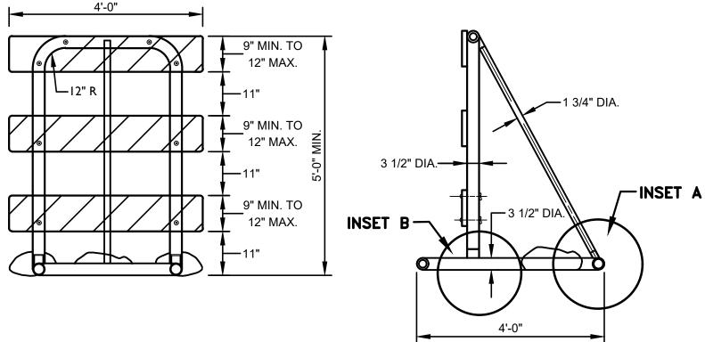
THE BASE AND UPRIGHT SHALL BE 3 1/2" DIA. ROTATIONALLY MOLDED POLYETHYLENE PLASTIC CONFORMING TO ASTM D 1248-II A3-E4. THE BRACE SHALL BE 1 3/4" DIA. EXTRUDED POLYETHYLENE PLASTIC CONFORMING TO ASTM D 1248-III A4. POLYETHYLENE PLASTIC SHALL BE WHITE AND SHALL BE ULTRA-VIOLET LIGHT STABILIZED.
